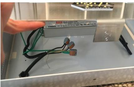
Figure 3: Connected wires inside bac of fixture.
